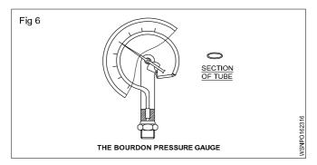
In I.C. Engines, Bourdon tube pressure gauges are widely employed for measurement of pressure, temperature and vacuum. In these gauges, a Bourdon tube which is a tempered, one is used and it attempts to straighten out under pressure and temperature and contact under vacuum.
