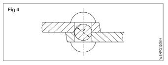
Rivet cross-section is the hole cross-section.
