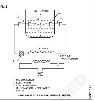
According to ISI specifications, the oil should be able to withstand 40 kV for one minute with a gap (4 mm  $\pm$  0.02 mm) between the electrodes and with the diameter of the electrodes as 13 mm.
